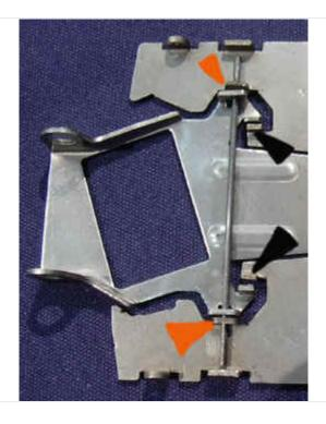
E2.3.8 JK X32 chassis for Super Production: The 64mm width regulation applies in these classes. Due to the manufacturing techniques, chassis may be delivered with the pan spread slightly at the rear so as to exceed the 64mm limit. The following methods only, are permitted to rectify this:
