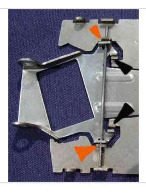
E2.3.8 JK X32 chassis for Super Production: The 64mm width regulation applies in these classes. Due to the manufacturing techniques, chassis may be delivered with the pan spread slightly at the rear so as to exceed the 64mm limit. The following methods only, are permitted to rectify this: Any or all of;
