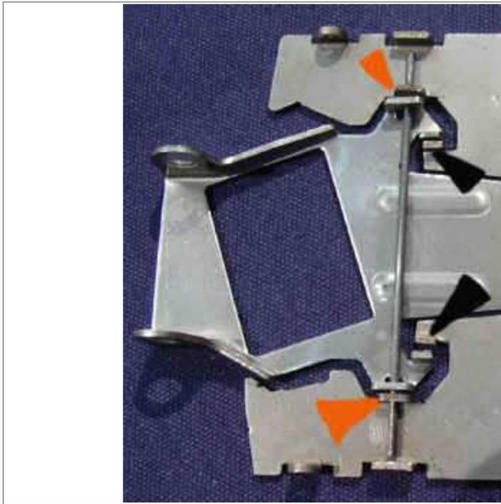
E2.3.8 JK X32 chassis for Super Production : The 64mm width regulation applies in these classes. Due to the manufacturing techniques, chassis may be delivered with the pan spread slightly at the rear so as to exceed the 64mm limit. The following methods only, are permitted to rectify this:
