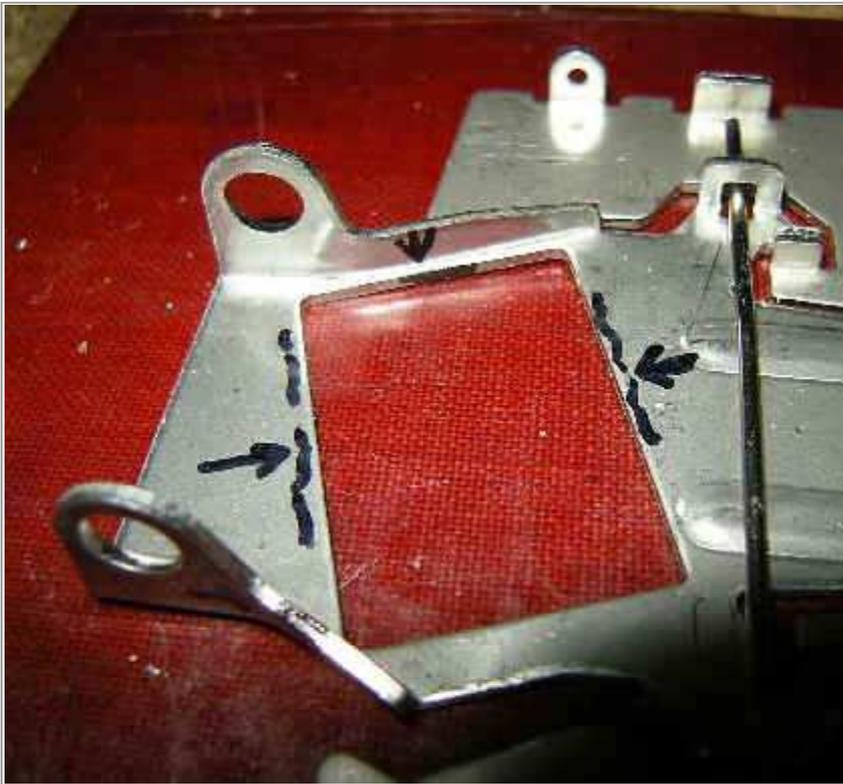
E2.3.7 JK X32 chassis for Super Production class: A small amount of material may be removed to facilitate installation of Wasp/Hornet Super Production motors as follows
