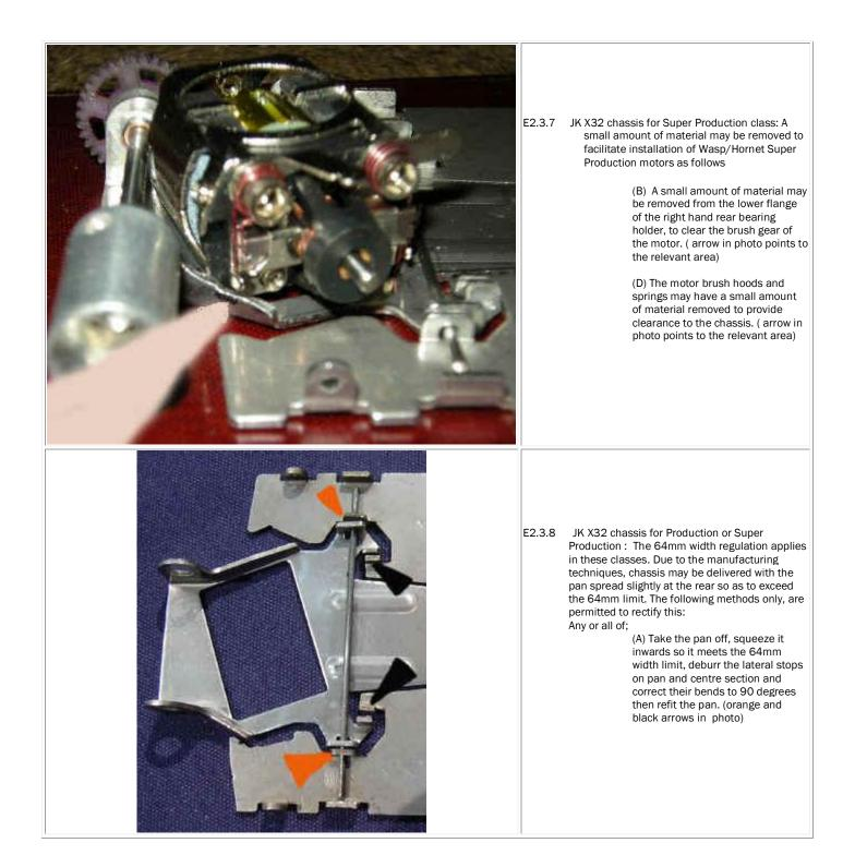
(B) A small amount of material may be removed from the lower flange of the right hand rear bearing holder, to clear the brush gear of the motor. (See illustrations)
