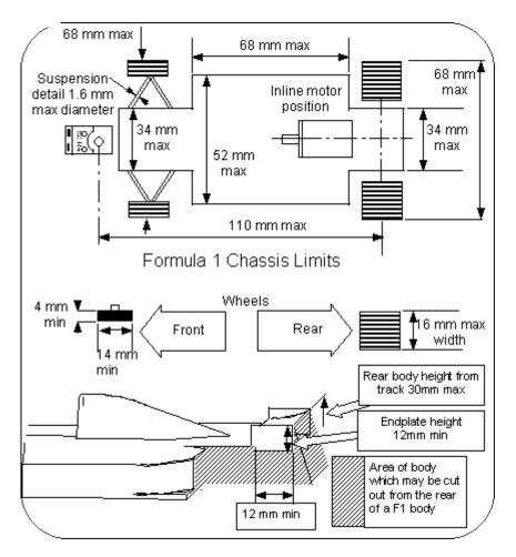
B5. Vacuum formed plastic bodyshells only are permitted and these shall not exceed 1 mm in thickness at any point. No weights may be attached to the body so as to be outside the chassis width limit. The diagram above shows what can be cut out.
