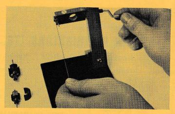
THE MINIATURE ARMATURE WINDING TOOL THAT ENABLES THE NOVICE TO COMPETE WITH THE EXPERT TO TAKE  $\frac{3}{8}$ ",  $\frac{1}{2}$ " and  $\frac{5}{8}$ " DIAMETER ARMATURES
