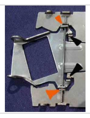
E2.3.8 JK X32 chassis for Production or Super Production: The 64mm width regulation applies in these classes. Due to the manufacturing techniques, chassis may be delivered with the pan spread slightly at the rear so as to exceed the 64mm limit. The following methods only, are permitted to rectify this:
